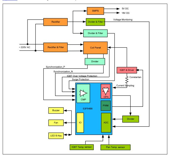
Figure 2-1 Block Diagram of IH Cooker System
